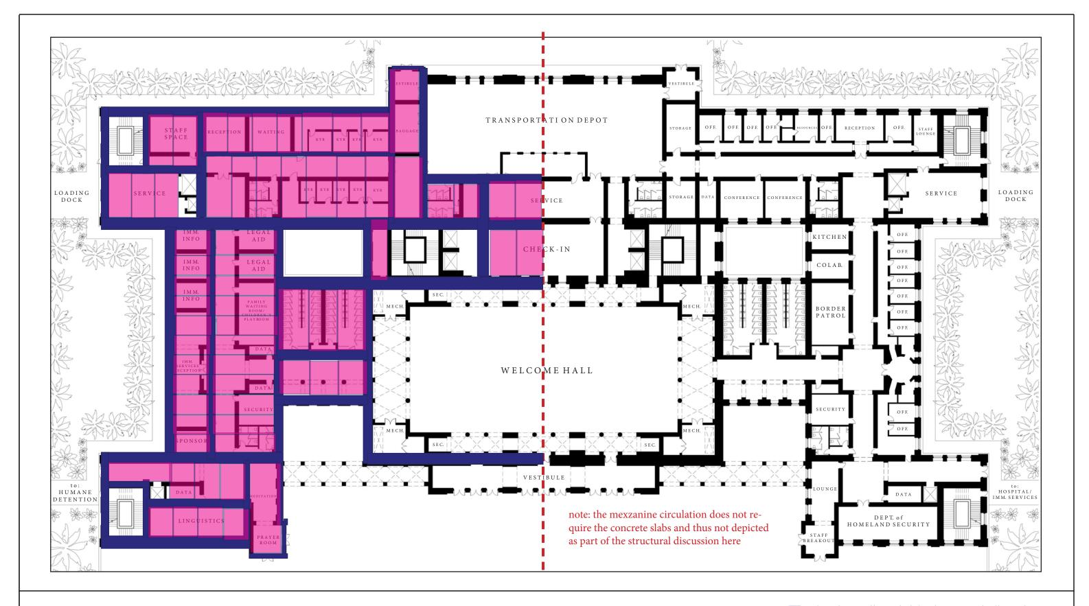
STRUCTURAL LAYOUT (8" hollow core concrete slab and stone masonry construction)
